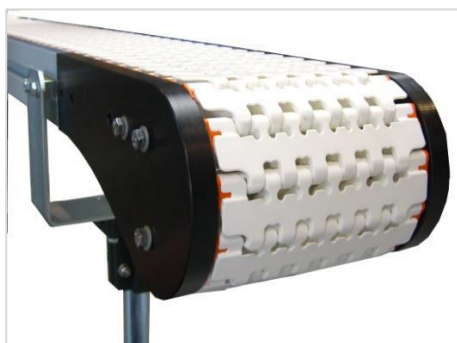
Fig. 3: Assembling the modular chain belt
